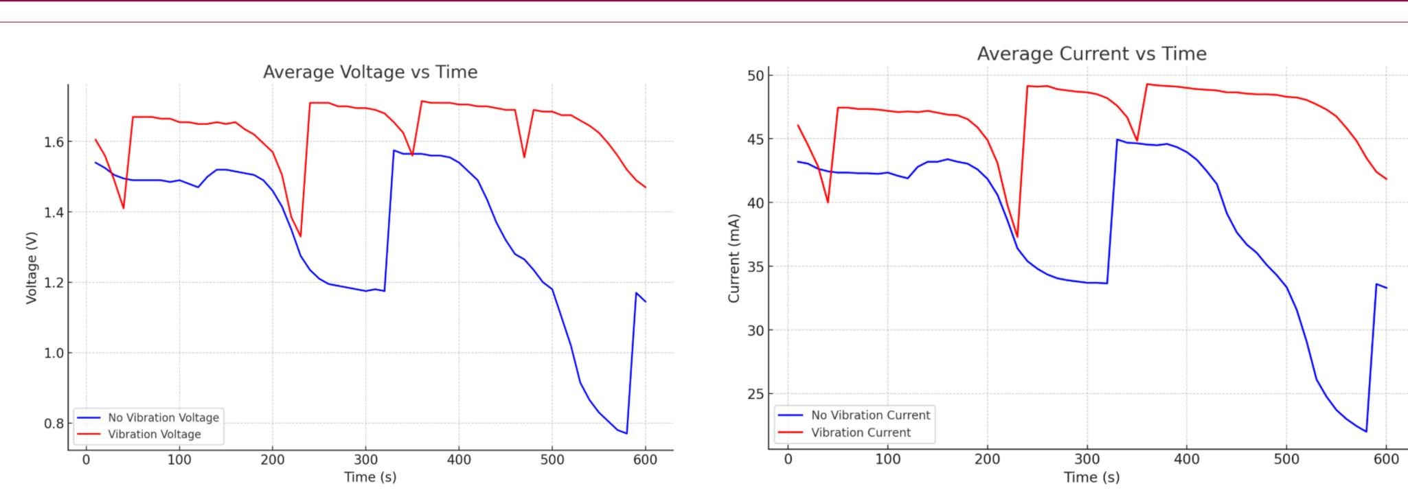
The voltage output from the fuel cell under vibration conditions consistently remains higher and more stable than the voltage under no vibration throughout the 600-second duration. The flow of water out of the battery affected the voltage greatly which is indicated by the sharp declines in voltage.
